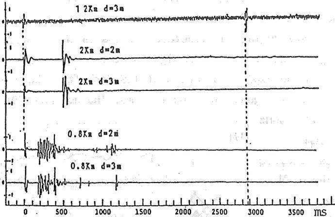
Fig.6 The EM received at the three stations after underground nuclear explosion ( 0.8Km, 2Km, 12Km)
