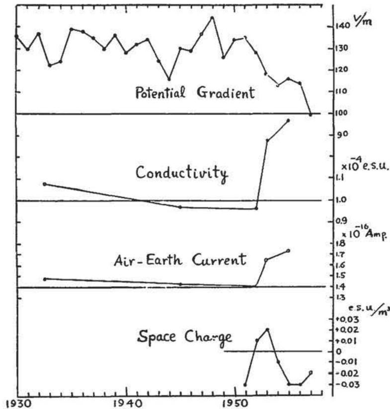
Fig. 1. The secular variations of the atmospheric electric elements observed at Kakioka.
