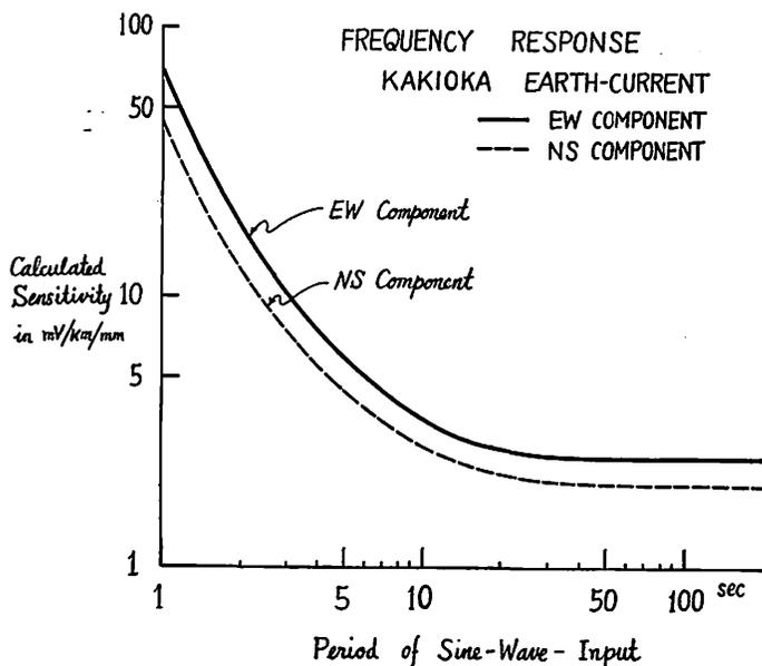
Fig. 5. (d) Sensitivities of the quick-run tellurigraph at Kakioka.
