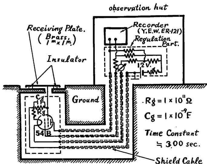
Fig. 1. Equipment of air-earth current measurement.
