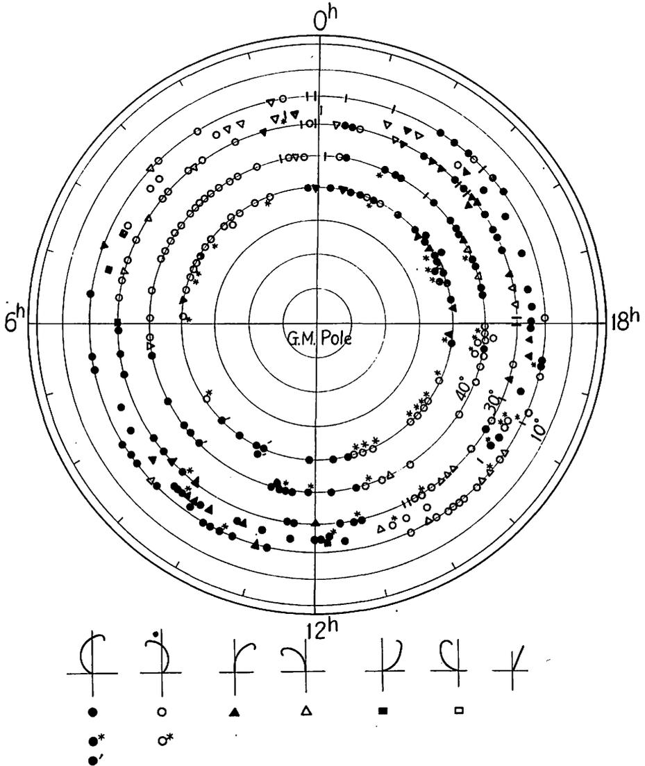
Fig. 16. Occurrence distribution of ssc's of such types as shown at the bottom of the figure in low and middle latitudes. Indications of each type are shown below each diagram, but ones appended by star, \*, or a dash, ', are of SSC\* or inverted SSC\*, respectively.
