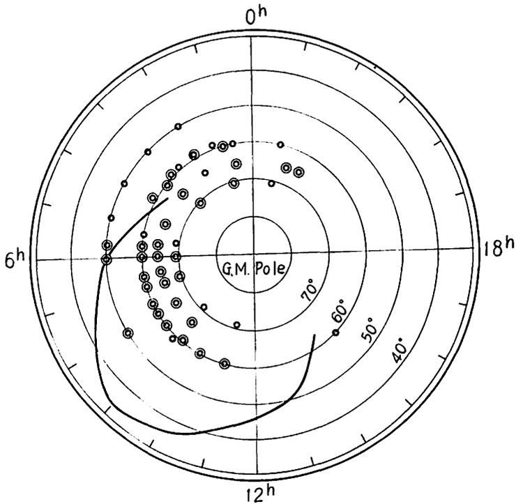
Fig. 14(b). Occurrence distribution of ssc's of Type B. The full line is the boundary of the occurrence region of ssc's of inverted SSC\* (SSC<sup>-</sup>), according to the Matsushita's result.
