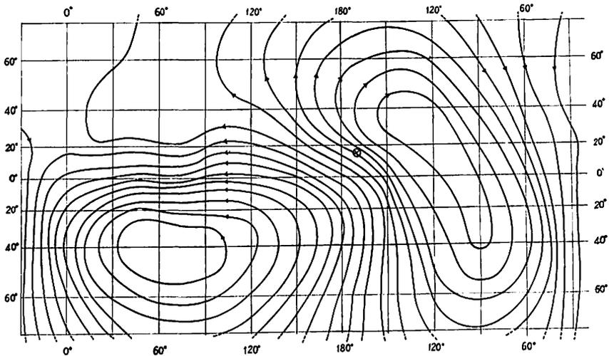
Fig. 4. The equivalent current system for the geomagnetic disturbances at 09h 02m, caused by the nuclear detonation on Johnston Island on July 9, 1962. The current of  $4.8 \times 10^3$  amp. flows between the adjacent stream lines.  $\otimes$  is Johnston Island.
