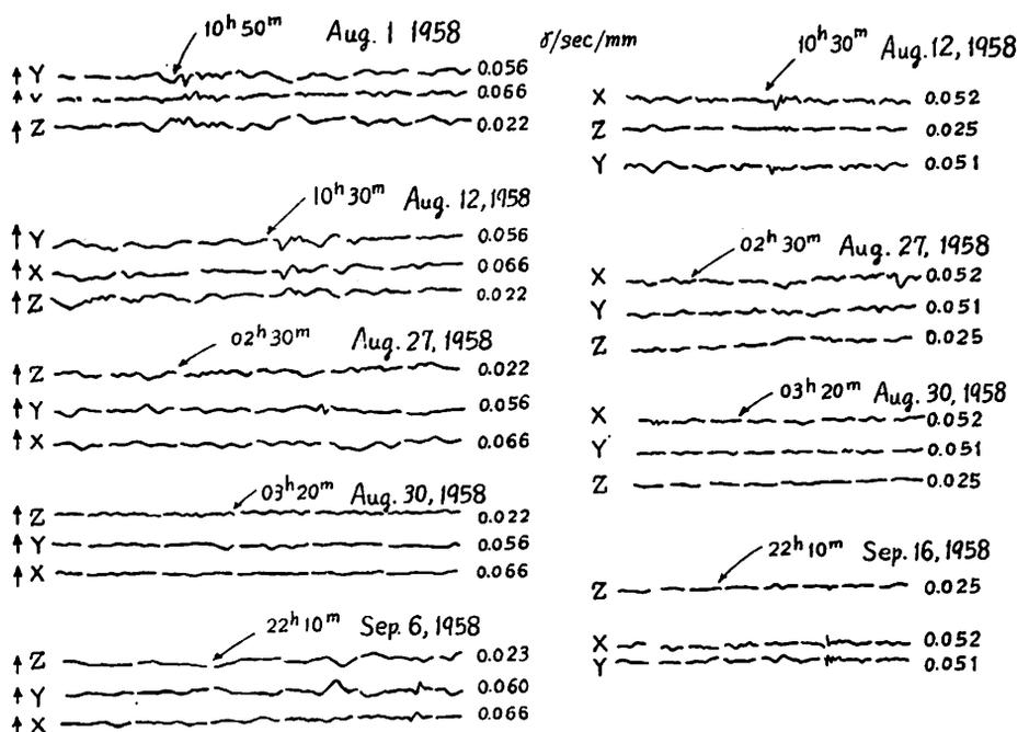
Fig. 1(b). Induction magnetograms at Memambetsu (Left) and at Kanoya (Right). One of Aug. 1, at Kanoya is a missing record. The scale values of the original records are given. On the original records, 1 minute is expressed by the length of 12 mm at Memambetsu and 6 mm at Kanoya.
