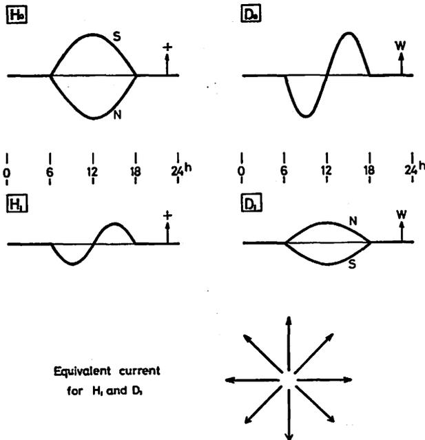
Fig. 5. Schematic diagram showing fundamental type of diurnal variation,  $H_0$  and  $D_0$ , and additional field,  $H_1$  and  $D_1$ . The lower figure is the equivalent current system for  $H_1$  and  $D_1$ .
