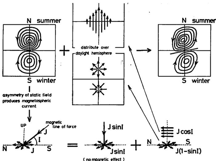
Fig. 6. A simplified model to account for the deformed Sq current vortex.
