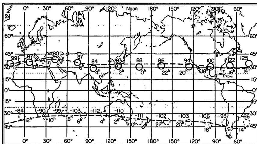
Fig. 2. Focus positions of  $Sq$  current system every two hours for the average of summer and winter during the Second Polar Year. Geographic coordinates. The number alongside each point indicates the potential (in units of  $0.825 \times 10^3$  cgs) at each UT epoch. The broken curves in the two hemispheres show the boundaries at which the harmonic coefficient  $a_1$  of diurnal component of the  $X$  variation changes its sign (after Hasegawa 1960).
