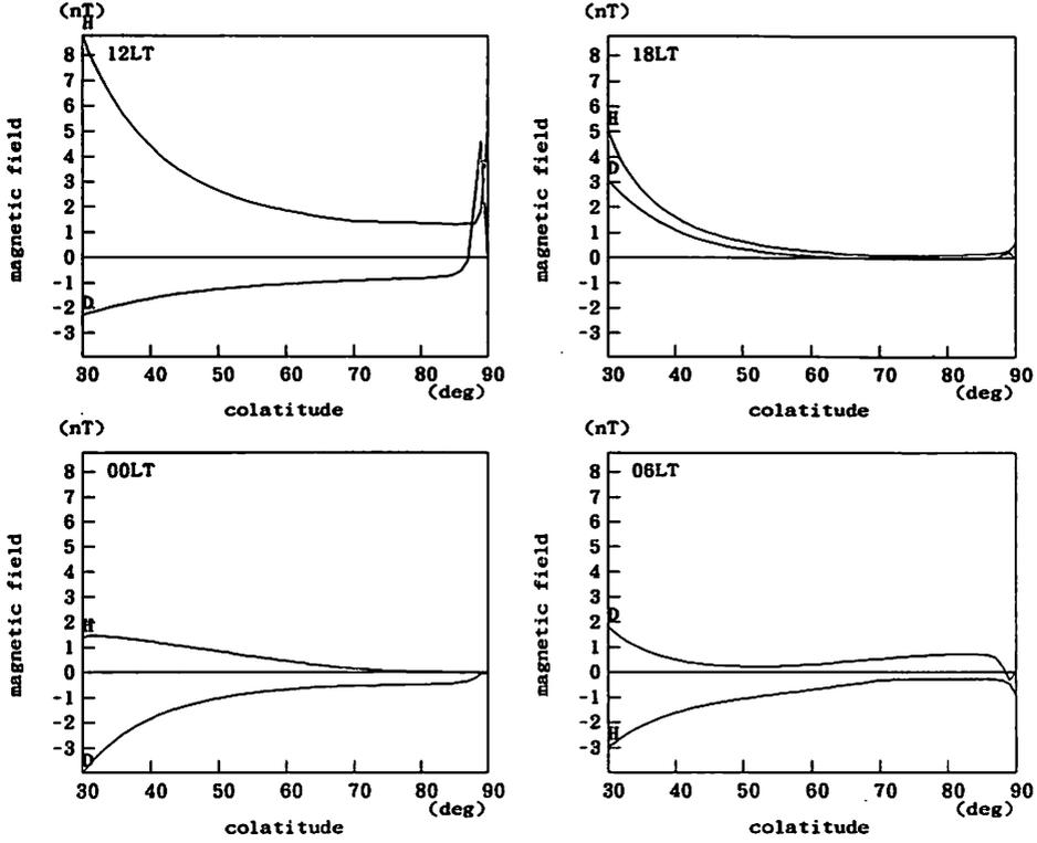
Fig. 10 Latitudinal variations of the two components of magnetic variations expected from model calculation of ionospheric currents for four local times.
