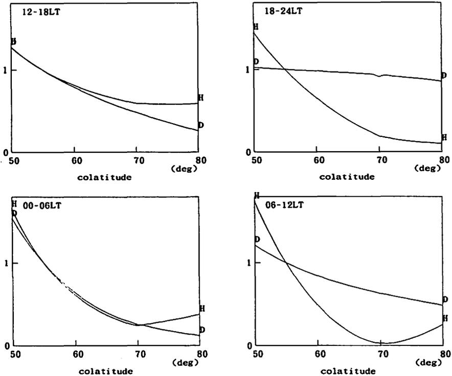
Fig. 11 Mean latitudinal variations of the two components of magnetic variations expected from the model calculation of ionospheric currents for four local time ranges. The values are normalized to that at 55 degree colatitude which corresponds to the magnetic dipole latitude of MMB.
