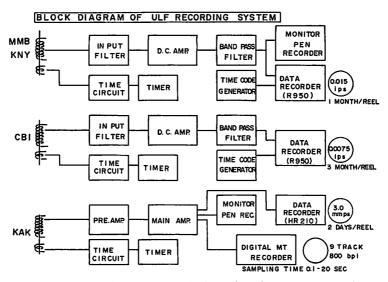
Fig. 1. Block diagram of pulsation observing systems at four observatories, Memambetsu, Kanoya, Chichijima and Kakioka.
